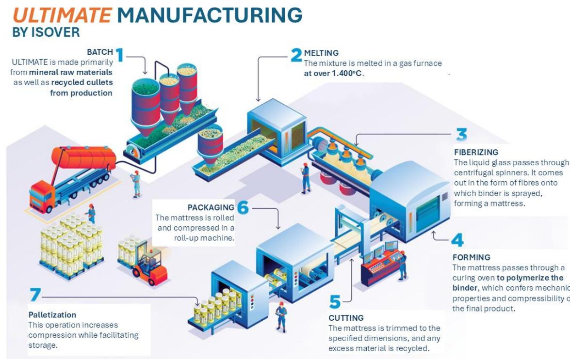
Mineral wool is made from high-temperature molten glass that is blown away using centrifugal force to form fine cotton-like fibers. Then, a binder is sprayed on the material to form it, and the product is heated in an oven. Hereafter, the product is cut to size and packed.
